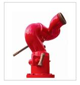
The single 4" full-flow waterway with internal turning vanes is designed to provide maximum efficiency at a maximum flow of 2,000 gpm (7,570 Lpm).
